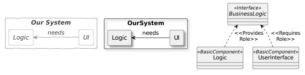
(a) Hand-drawn sketch (b) Machine readable diagram (c) Visualized Architecture Model
