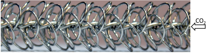
Figure 3.7: Image of the hiTRAN ® wire matrix element applied in the test section. The flow direction against the inclined windings is indicated by the arrow.
