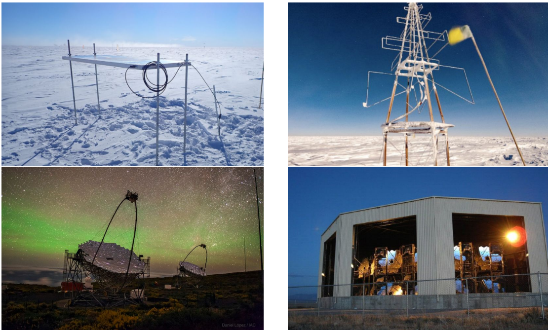
Figure 2.3.: Examples of deployed detectors. A scintillation detector at the IceCube Neutrino Observatory (upper left), a Radio detector at the IceCube Neutrino Observatory (upper right), an air Cherenkov detector Major Atmospheric Gamma Imaging Cherenkov Telescopes (downleft) and the Fluorescence detector at the Telescope Array experiment (downright) [16, 17, 18, 19].
