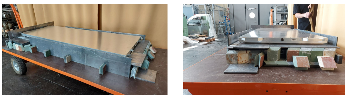
Figure 5.7.: Experimental setup with neutron and gamma shielding for the measurements done in 2022.
