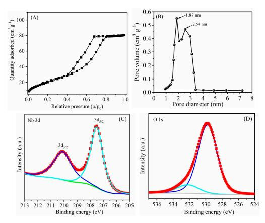
**Figure 4.** (**A**) Nitrogen adsorption-desorption isotherm at 77 K and (**B**) BJH pore size distribution analysis of  $T-Nb_2O_5$ . High-resolution XPS spectra of (**C**) Nb 3d and (**D**) O 1s for the  $T-Nb_2O_5$ .
