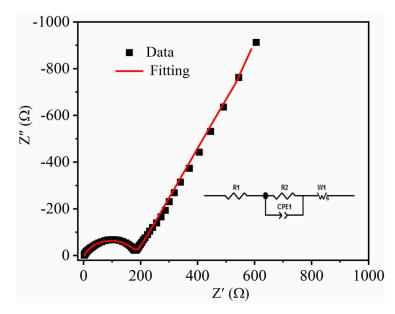
Figure 7. EIS Nyquist plots of the T–Nb<sub>2</sub>O<sub>5</sub> electrode.
