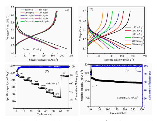
**Figure 6.** (**A**) Typical charging-discharging profiles at 100 mA  $g^{-1}$  for the first ten cycles, (**B**) the charging and discharging curves at different current rates, (**C**) the rate performance, and (**D**) the cycle performance at 250 mA  $g^{-1}$  for the T-Nb<sub>2</sub>O<sub>5</sub> electrode.
