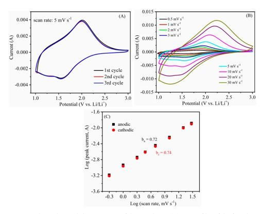
**Figure 5.** Electrochemical characteristics of the  $T-Nb_2O_5$ : (**A**) CV profiles of the first three cycles; (**B**) CV profiles at different sweep rates ranging from 0.5 to 30 mV s<sup>-1</sup>, and (**C**) corresponding logarithmic relationships between the scan rates and peak currents.
