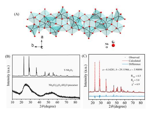
**Figure 2.** (A) Crystallographic structures of  $T-Nb_2O_5$  (orthorhombic, S.G. *Pbam*); (B) Comparison of XRD patterns of  $Nb_2(O_2)_2O_3 \cdot 6H_2O$  precursor and  $T-Nb_2O_5$ . (C) Rietveld refined XRD pattern of the  $T-Nb_2O_5$ .
