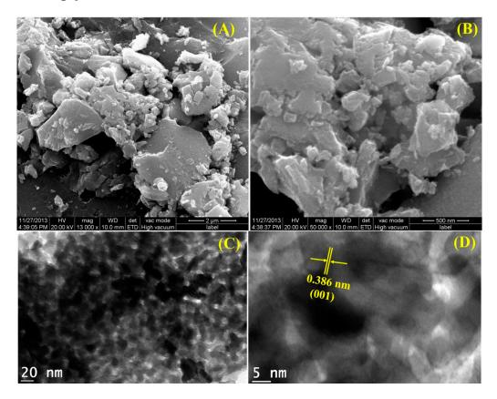
Figure 3. Different magnified SEM (A,B) and TEM (C,D) images of orthorhombic T–Nb<sub>2</sub>O<sub>5</sub>.
