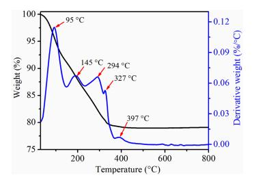
Figure 1. TGA and DTA of the as-synthesized peroxo niobic acid sol precursor.
