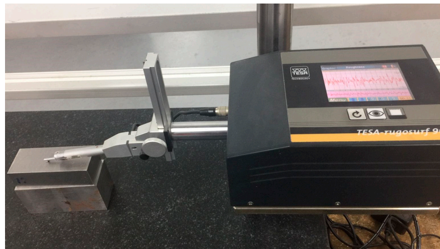
Figure 4. Setup for evaluating surface roughness quality of milled samples.
