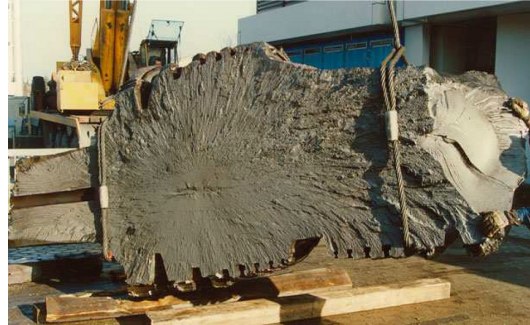
Figure 1.3.: Fragment of Irsching burst steam turbine rotor. There were no fatalities [2].
