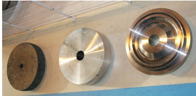
Figure 1.4: Heavy-duty gas turbine rotor disk forgings at different manufacturing stages: after forging and heat treatment (left), ultrasonic contour (middle), rough machining contour (right). From Zimmer et al. [111].
