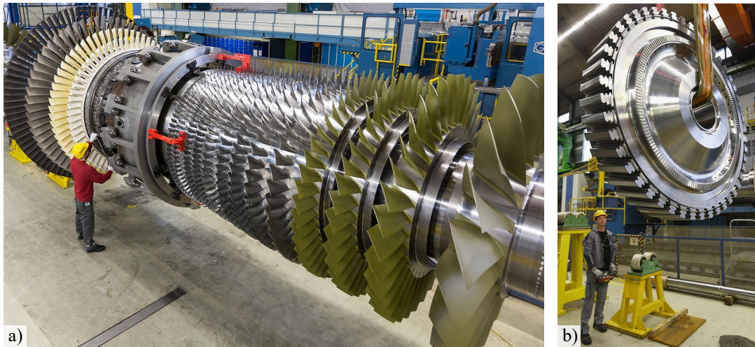
Figure 1.1.: (a) Assembly of the SGT5-8000H at the Siemens Energy gas turbine plant in Berlin. (b) A worker with a finished disk for a gas turbine. With permission by Siemens Energy.
