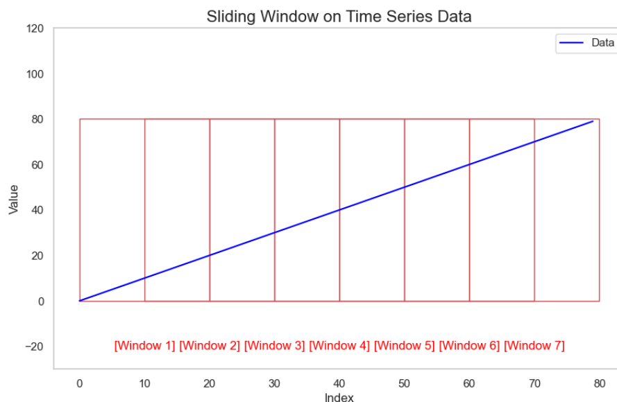
Figure 3.1: A sketch of sliding window on time series data with a window size of 20 and a window stride of 10.
