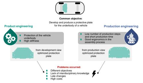
**Figure 2** Example of the development and production of a protective plate for the underbody of a vehicle and problems that occur during the engineering process
