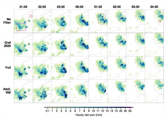
**Figure 4.** Maps of a rainfall event (21 June, 21:50 to 22 June, 4:50) (time progressing from left to right). The first three rows are interpolations based on commercial microwave links for the different processing lines. The bottom row is the reference RADOLAN-RW. A comparison of the *Full* processing and RADOLAN-RW in a movie sequence can be found in Blettner (2023).
