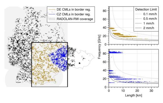
**Figure 1.** Data overview. Left: Sensor locations with the analyzed border region defined by the black box; the shaded background shows the coverage of RADOLAN-RW. Right: Distribution of frequency versus length of commercial microwave links (CMLs) within the analyzed region (German and Czech CMLs in upper and lower panel, respectively); dashed lines show levels of detection limit.
