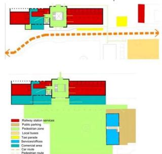
Figure 5: Station working schemes. First floor. Source: Prepared by the author
