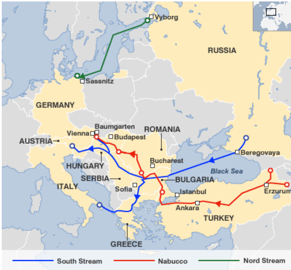
Figure 8 : Nordstream, Nabucco, and South Stream Pipeline Routes.
