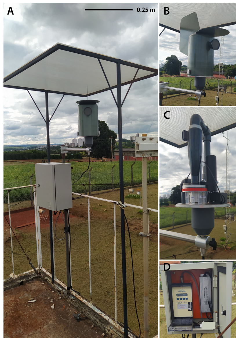
Figure 1. (A) High-volume cyclone air sampler from Agri Samplers Ltd., (High Wycombe, UK), with a protective roof designed, built and attached to the top of the equipment, installed in Londrina, PR, operating at the IDR—Paraná (Paraná Agricultural Development Institute, Londrina, Brazil) Experimental Station. (B) Front view of the sampler unit mounted with a wind-driven wing, installed within the limits of a weather station in the background. (C) Details of the uncovered spore sampler unit and (D) control panel by which sampler parameters are defined. 1 Pictures from A.A.P.Custódio. 1 The device samples a high volume of air (270 L per minute), which is 27 times more than the traditional Burkard seven-day spore trap. Spores are also collected directly into tubes to facilitate easy lab-based processing. The figure (A) shows important adaptations built by our aerobiology research group for its use in Brazil to protect it from the extremes of the sun and heavy rain, and to raise it into more mobile air-flow, which improves the representation of the sample to the wider region.
