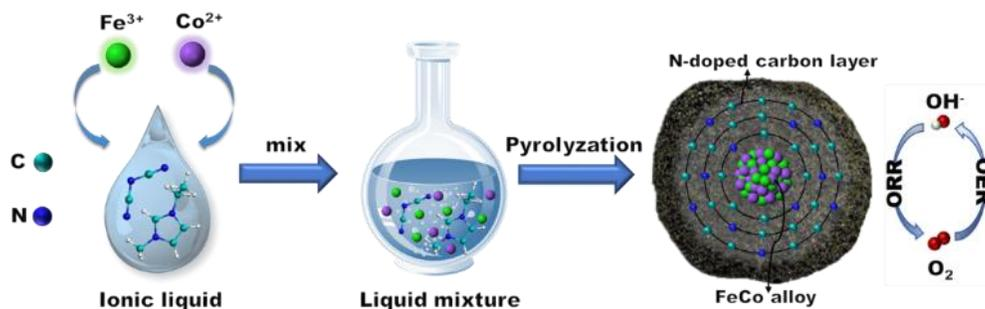
Figure 4.1 Synthesis process of FeCo@NC,
