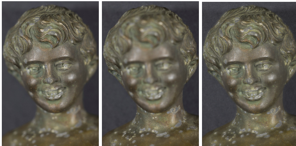
Figure 3. Different images from the image stack. Only the information of the regions in focus are used for the 3D reconstruction.
