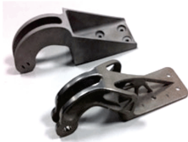
A 50% lighter prototype jet engine part made by additive manufacturing (front) www.ipmd.net
