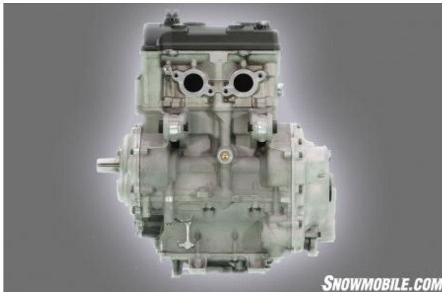
Figure 4: Yamaha Genesis 80FI engine from snowmobile.com
