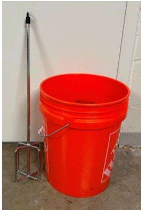
Figure 4. Eggbeater and bucket mixer intended for full-brick production
