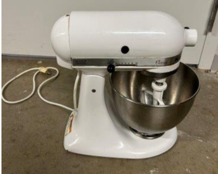
Figure 3. KitchenAid stand mixer used for producing concrete coupons
