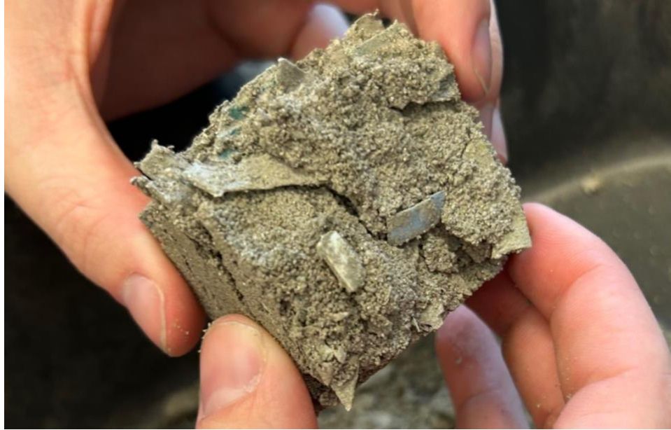
Figure 13. Plastic distribution of concrete coupon post-compressive testing
