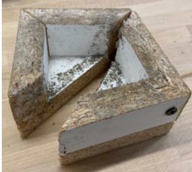
Figure 6. Melamine coated wood mold for concrete coupons.
