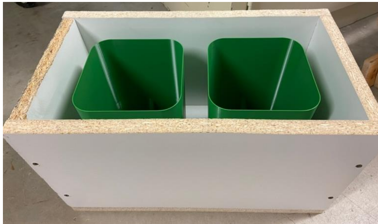
Figure 7: Melamine mold intended for full-size concrete bricks
