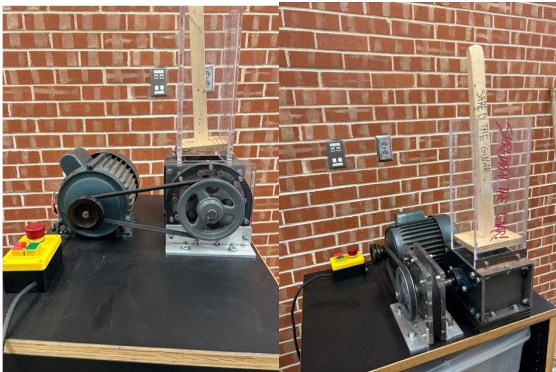
Figure 1: Side and front view of the shredder with the plunger inserted.
