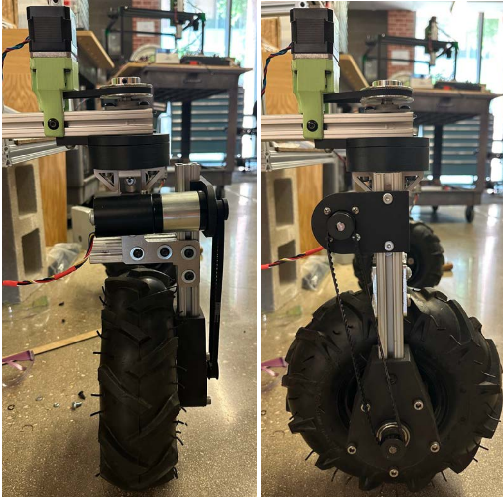
Figure 5: Fully Constructed Steering Column
