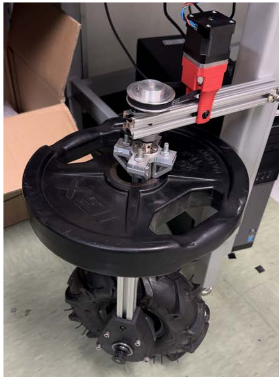
Figure 12: Final steering motor assembly test setup
