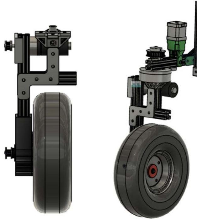
Figure E9: Steering column assembly before (left) and after (right) mounting to the main rover body with the 3D printed supports
