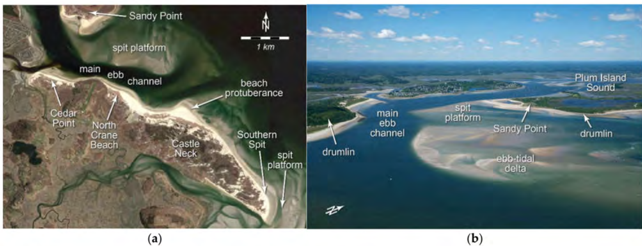
Figure 6. Morphological components of the Plum Island Sound Inlet sand-bypassing system. (a) Landsat satellite image from 14 April 2017. (b) Oblique aerial photo looking west into Plum Island Sound Inlet.
