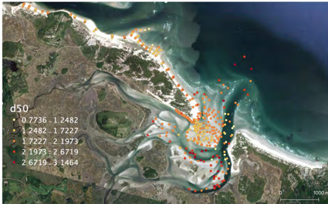
Figure 5. Grain-size trends along Castle Neck and at Essex Inlet (grain size in phi). Note the general decrease in grain size (increasing phi value) toward the inlet and into Essex Bay.
