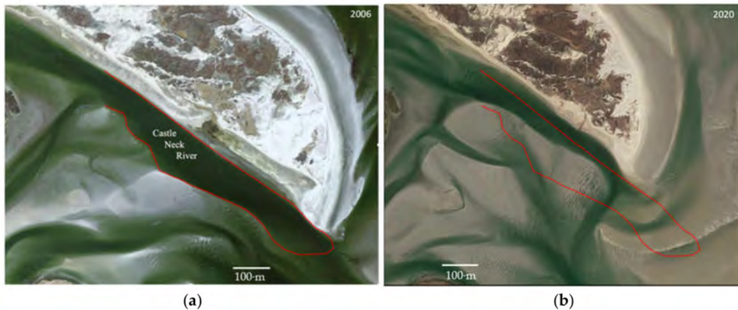
Figure 13. Changing morphology of Castle Neck River (outlined in red) behind Southern Spit, illustrating sand infilling between (a) 2008 (MassGIS) and (b) 2019 (Landsat Copernicus).
