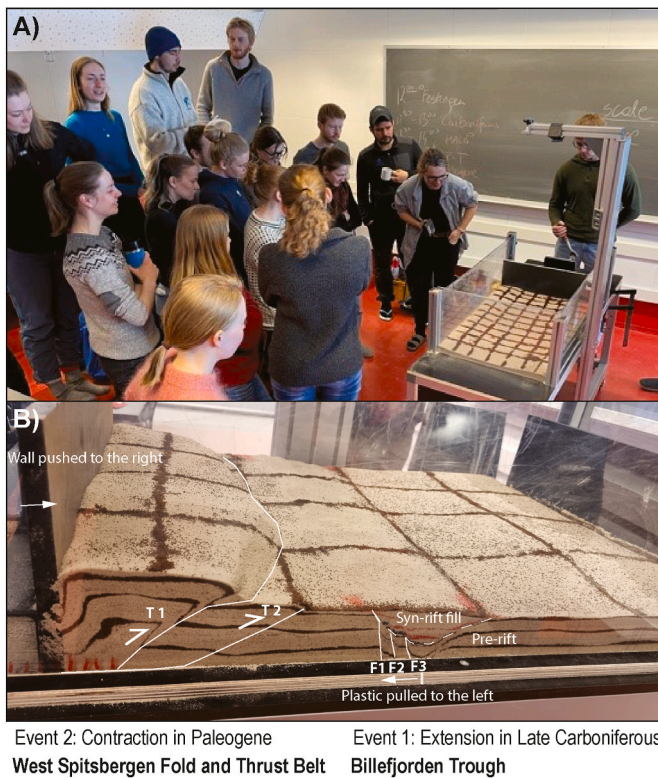
Fig. 14. Illustration of using a qualitative sandbox model during structural geology teaching at UNIS. A) Students of the AG209 course on the “Tectonic and Sedimentary History of Svalbard” discussing a compressional experiment using the UNIS in-house Svalbox sandbox model. B) Detailed view of some of the generated compressional features.
