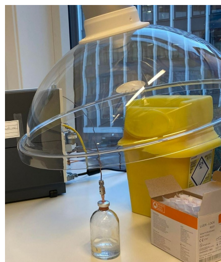
(b) Illustration of gas composition measurements using a microGC.
