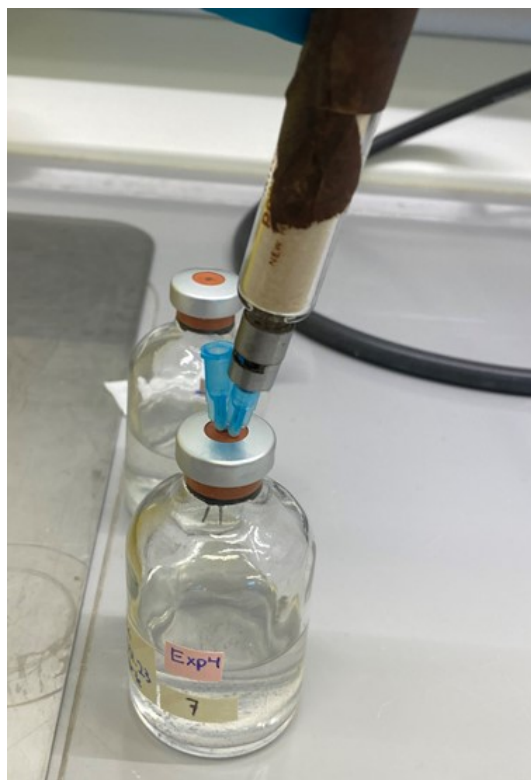
Figure 3.2: Illustration of how the gas line method is flushing the bottle using a needle connected to the gas line and a disconnected needle to exchange the gas composition.
