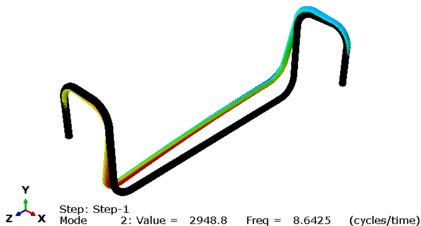
Figure 7.4: Mode one of the Z-shaped jumper. Displacement in the x-direction
