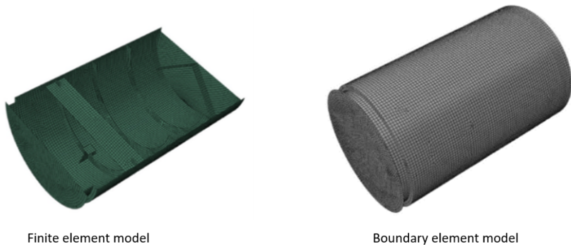
Figure 3.5: The finite and boundary element model of the cylindrical shell, Gao et al. (2022) [61]
