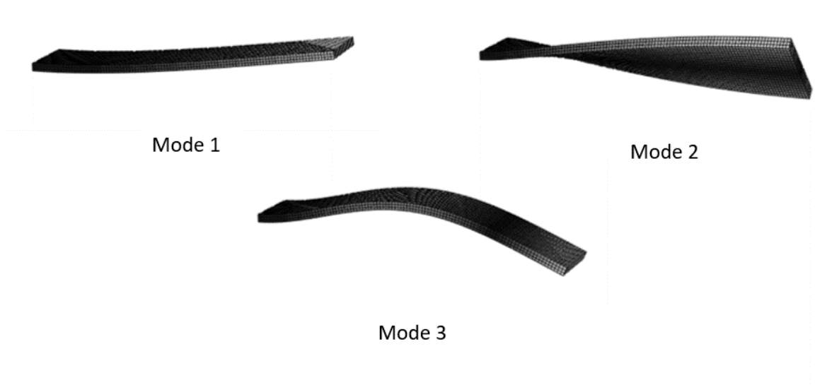
Figure 3.4: First three modes of submerged cantilever plates
