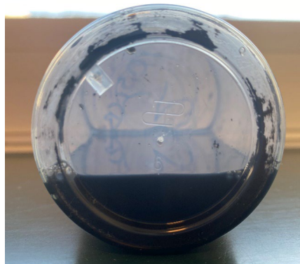
(c) Sedimentation on the container bottom after seven days (a sample was collected after the experiments)
