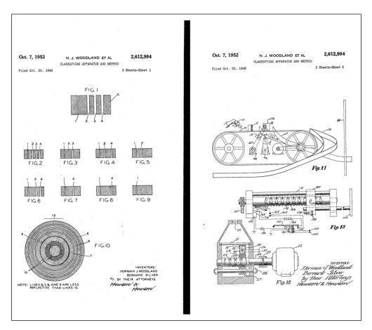
Figure 2. First two pages from Woodland and Silver's patent for a "Classifying apparatus and method" (1952), including schematics of the barcode and its reading apparatus.
