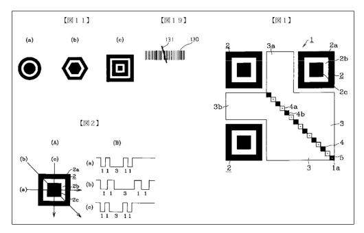
**Figure 4.** Illustrations from the "Two-dimensional code" patent (Hara et al., 1999) detailing shapes and positioning of the finder pattern around the main data area, as well as examples of how the 1:1:3:1:1 ratio remains constant across scanning orientations vis-à-vis the horizontal scanning of one-dimensional barcodes.
