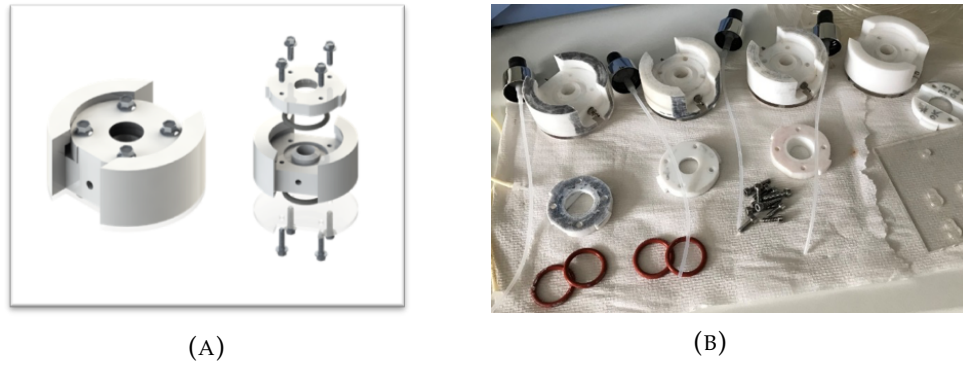
FIGURE 5.5: Perfusion module design and manufacturing. SOLIDWORKS renderings (A) and final prototypes manufactured in PTFE (B).
