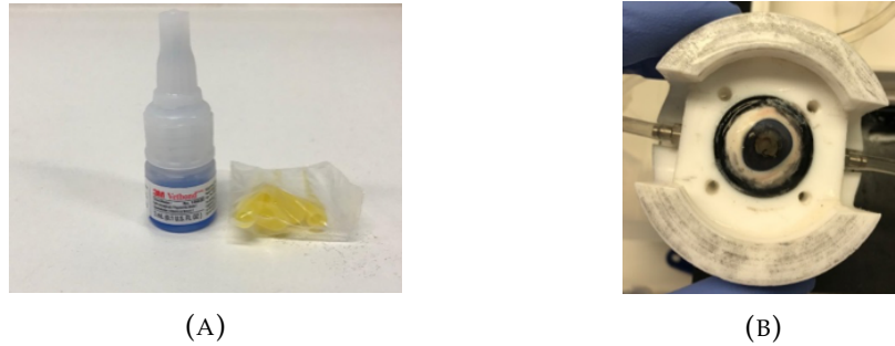
FIGURE 6.3: 3M TM Vetbond TM tissue adhesive (A); porcine anterior segment glued to the perfusion chamber (B).
