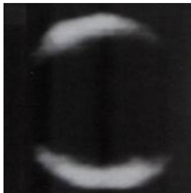
Figure 1.11. Evolution of ion imaging techniques. Vibrationless methyl \text{CH}_3(v=0) fragments images produced by projecting onto two dimensions the three-dimensional spatial distribution of products from photodissociation of \text{CH}_3\text{I} with 266 nm laser light. The plane of the projection is parallel to the polarization axis of the pump laser beam. Image obtained by Houston and Chandler in 1987. 36
