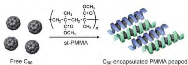
Figure 2.37 Encapsulation of C_{60} using a st-PMMA polymer.
