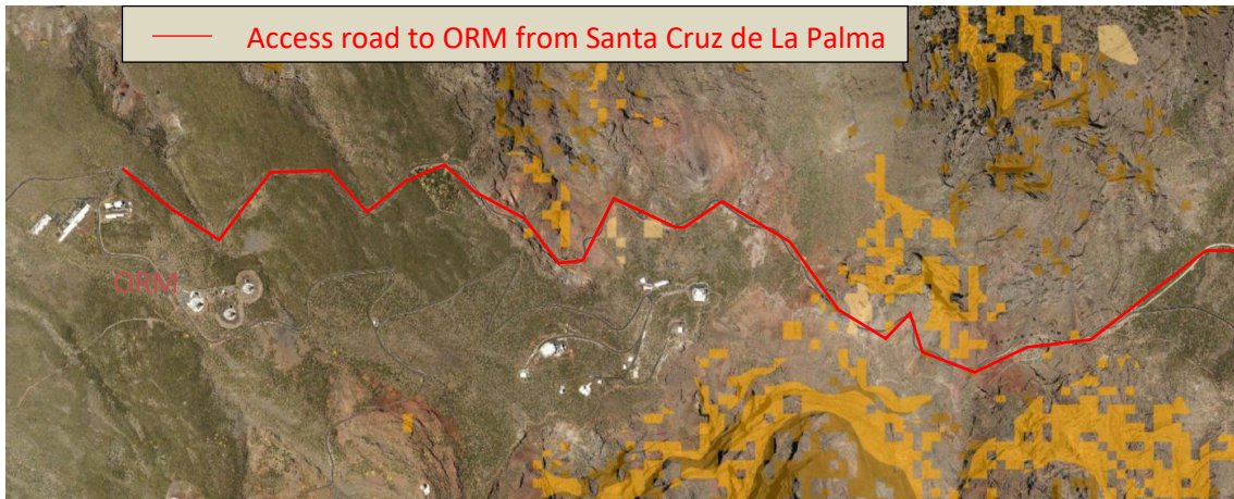
Fig. 2-30: Gravitational movement risks areas(yellow) in the access road to the ORM [16].
