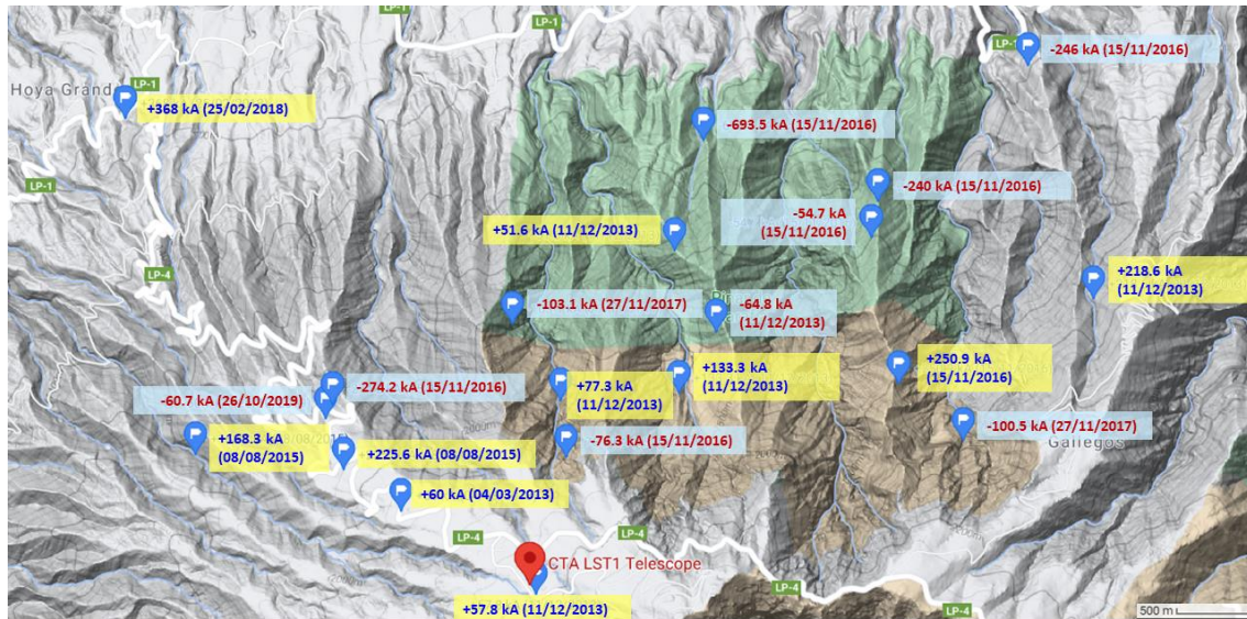
Fig. 2-19. Lightning strikes recorded by Vaisala GLD360 Network around LST1. Data correspond to events registered between 2013 and 2020. The image shows all the strikes registered within the square defined by corners 28^{\circ}47'42.0''N 17^{\circ}55'48.0''W and 28^{\circ}45'36.0''N 17^{\circ}51'00.0''W . Credits: Vaisala
