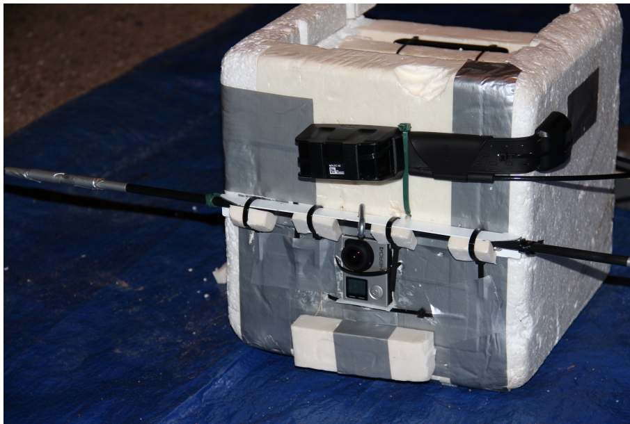
Figure 4.8: Detail of the bottom part of the probe for Daedalus 19 mission. The nadir port hosts a GoPro camera for light pollution research. Image provided by ORISON project.
