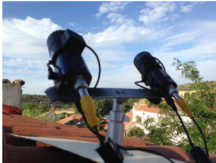
Figure A.1: Field test setup with both cameras using same lenses, framegrabbers and settings, and pointing to the same field of view.
