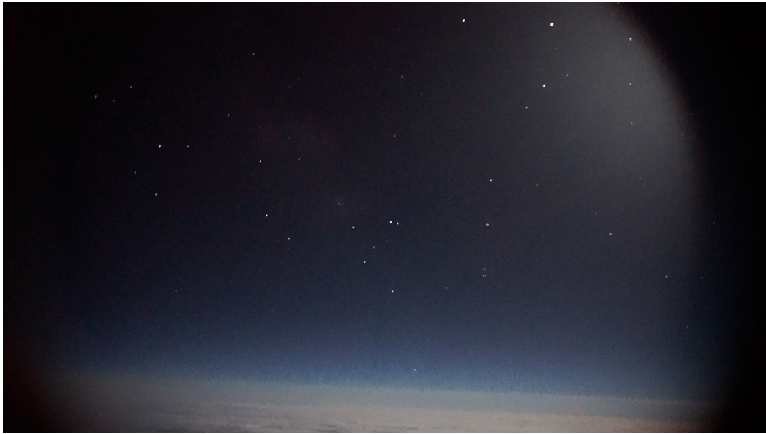
Figure 4.12: Sony \alpha 7S imaging Scorpio and Sagittarius constellation, showing stars up to magnitude 6.5. Galactic centre is also visible.
