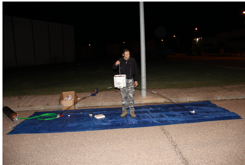
Figure 4.10: Probe configuration before launch of Daedalus 19, ready to attach the balloons. The probe has a long rod and the mass is distributed to increase the moment of inertia. Image provided by ORISON project.
