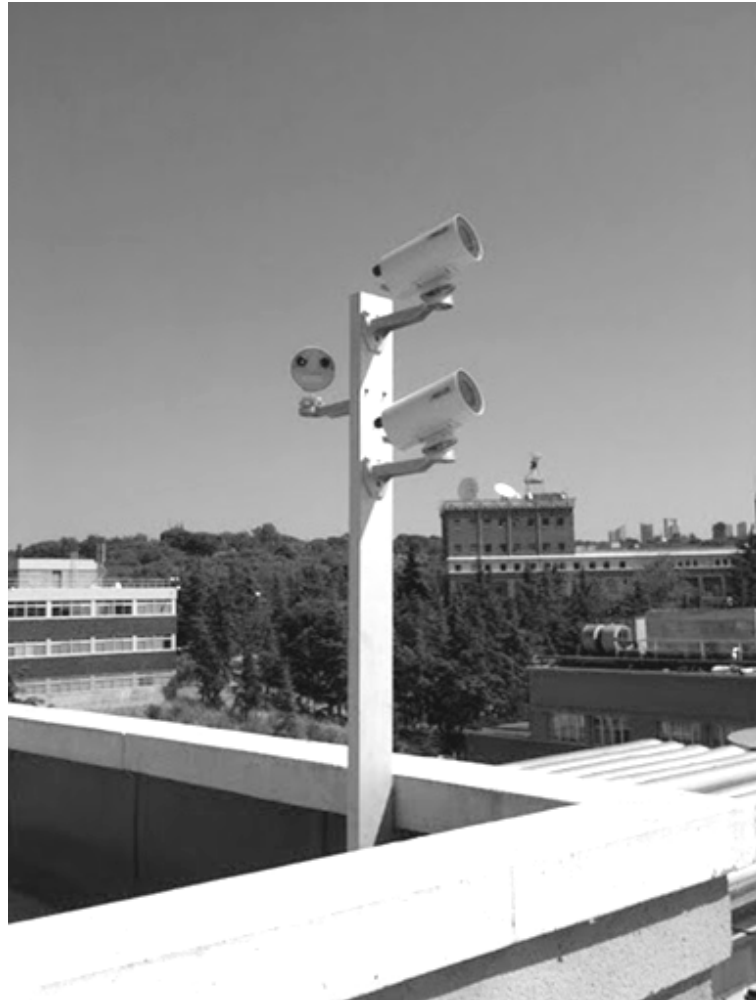
Figure 4.2: Actual appearance of the cameras mounted close to the Observatorio UCM domes. The cameras were distributed in three poles to avoid the appearance of the domes in the FoV.
