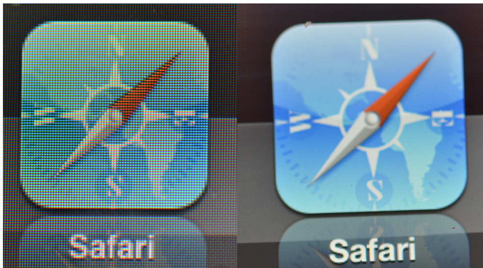
Figure 33 Anand Lal Shimpi, (2012), Ultra-High-Resolution Displays Physically Removes Aliasing [ONLINE]. Available at: https://www.anandtech.com/show/5655/physical-impressions-of-the-new-ipad-retina-display-shots [Accessed 12 February 2019].
