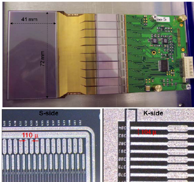
Figure 2.11: Photograph of a Micro-Stripped Double Sided Silicon Detector (DSSD), showing the 0.3 mm thick sensor and with two pictures zoomed to the readout area, indicating the readout pitch which is 110 \mu\text{m} and 104 \mu\text{m} for the S-side and K-side respectively. Image taken from [50].
