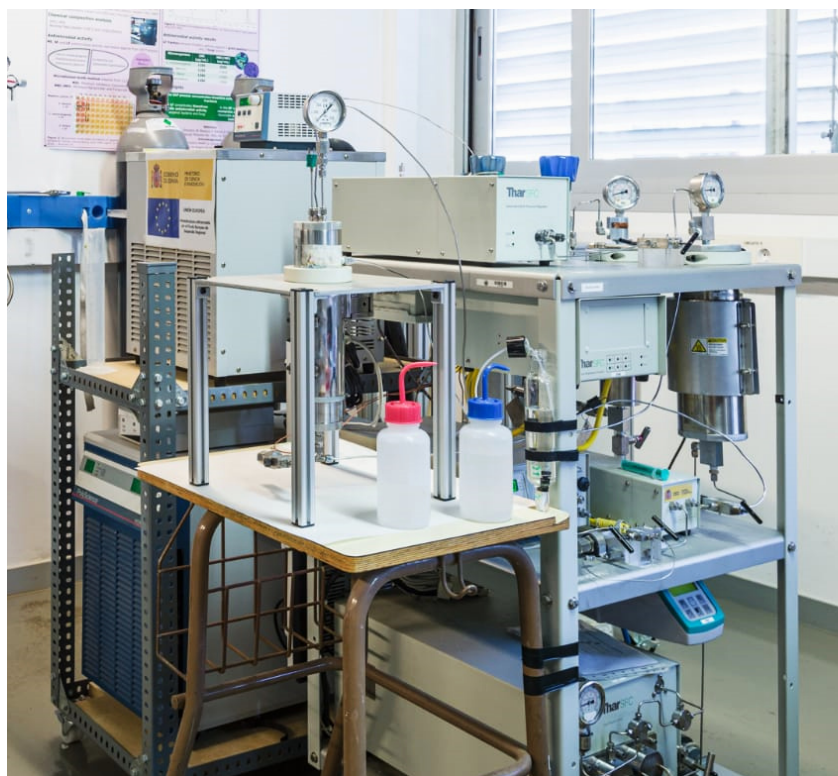
Figure III.4. Picture of the lab-scale Supercritical Anti-solvent Fractionation equipment located in the Green Chemistry Lab, I3A Institute, Zaragoza, Spain.
