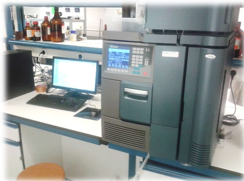
Figure III.8 HPLC Waters® Alliance 2695 equipment, PDA Waters®2998 detector and computer for the control and data processing.
