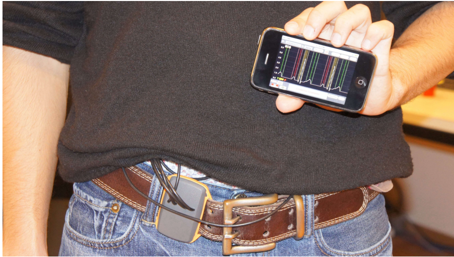
Figure 5.1: Electrode sensors on the skin link to the Shimmer™ platform clipped to a patient's belt sending continuous data to an iPhone, which displays the ECG signal, heart beat rate and delineation results
