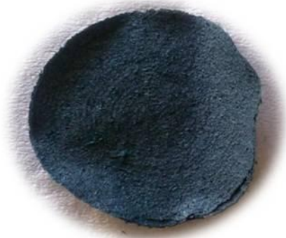
Figure 6.36. Entangled green sheet of \text{H}_2\text{V}_3\text{O}_8 obtained after 2 hours microwave irradiation.
