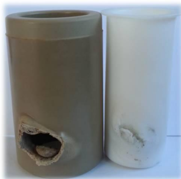
Figure 6.35. Catastrophic failure of a teflon vessel due to an uncontrolled formation of hot spots in the vessel walls during the synthesis of \text{H}_2\text{V}_3\text{O}_8
