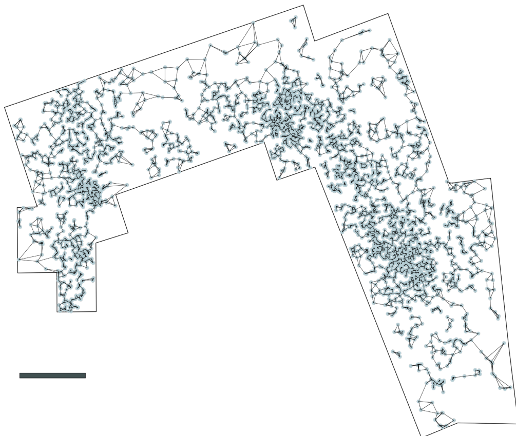
FIGURE 2.2. K -nearest neighbor graph of the DS point pattern generated with a K value of 3. Scale: 5 meters.
