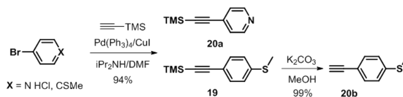
Scheme 15: Synthetic procedure towards 4-[(trimethylsilyl)ethynyl]pyridine 20a and (4-ethynylphenyl)(methyl)sulfane 20b .
