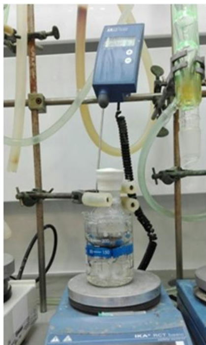
Figure 84: “Unconventional” system to avoid the folding of the Cu-supports.
