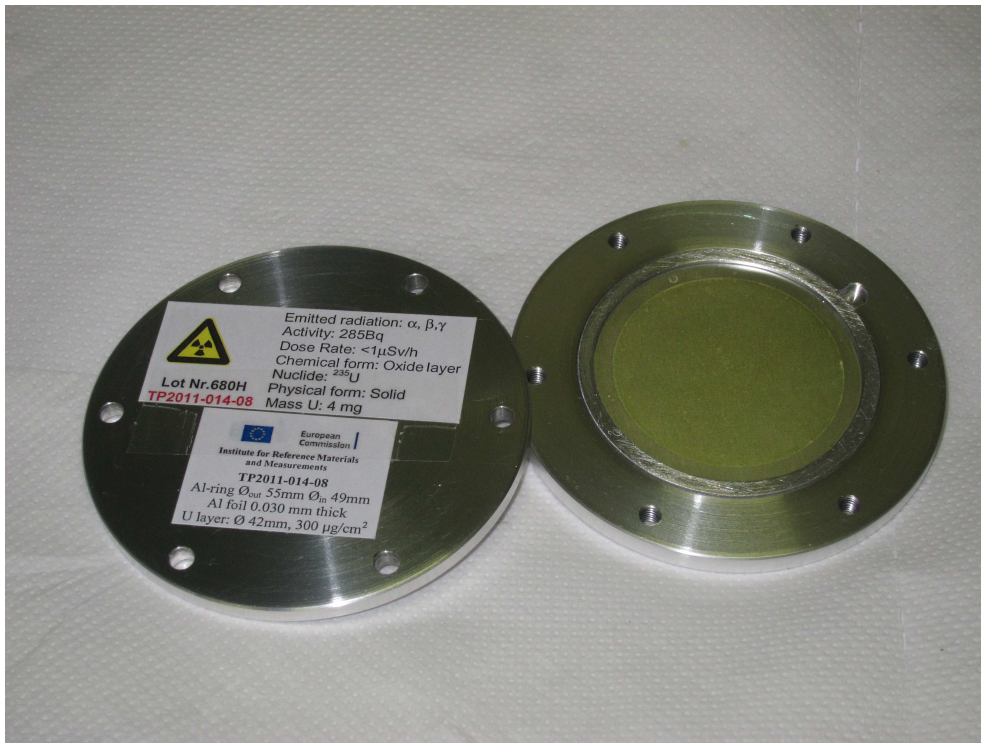
Figure 2.13: One of the ten ^{235}\text{U} samples used for the measurement of the ^{235}\text{U}(n,\gamma) cross section.
