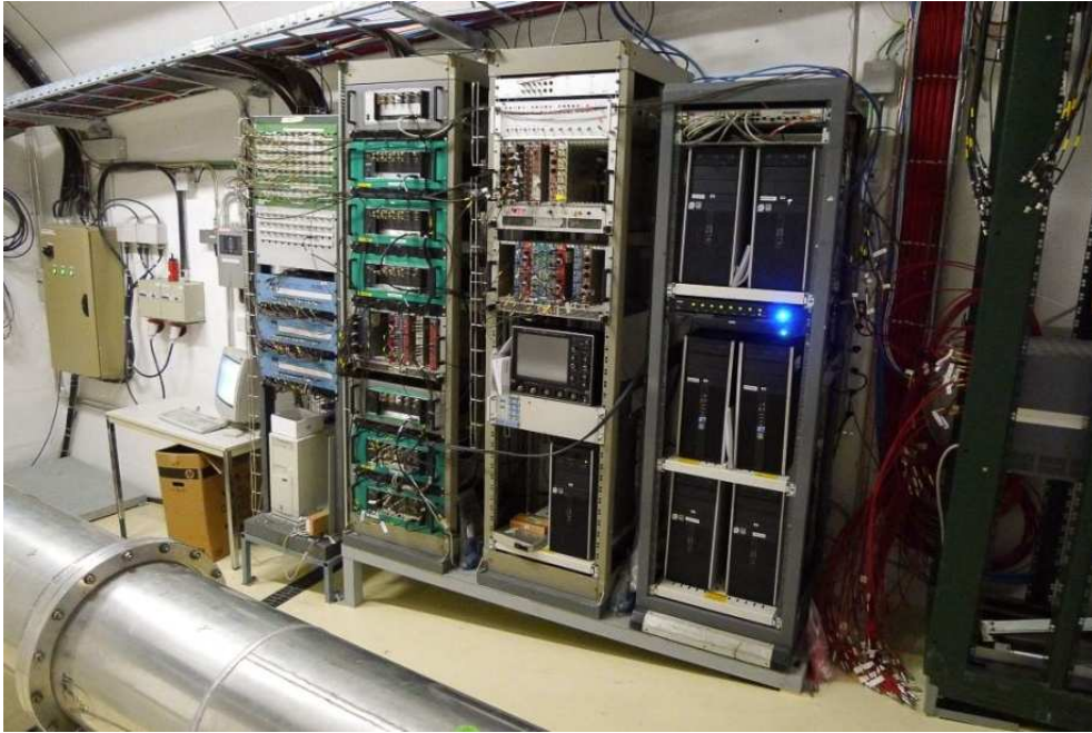
Figure 2.12: Front-end n_TOF DAQ formed by the Acqiris-DC270 flash ADCs cards used for the digitization of the signals of the detectors placed in the experimental area 1 (EAR1).
