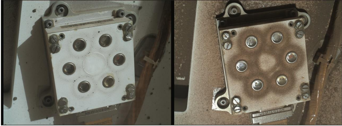
Figure 10.3. MAHLI images of the REMS UVS on sols 36 (left) and 1314 (right). A significant amount of dust has been deposited on the sensor, especially around the circular magnets that surround each photodiode.
