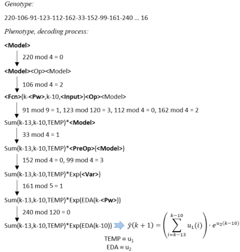
Figure A.5: Decoding process in GE that, starting from the genotype above, obtains the phenotype by mapping through the proposed grammar.
