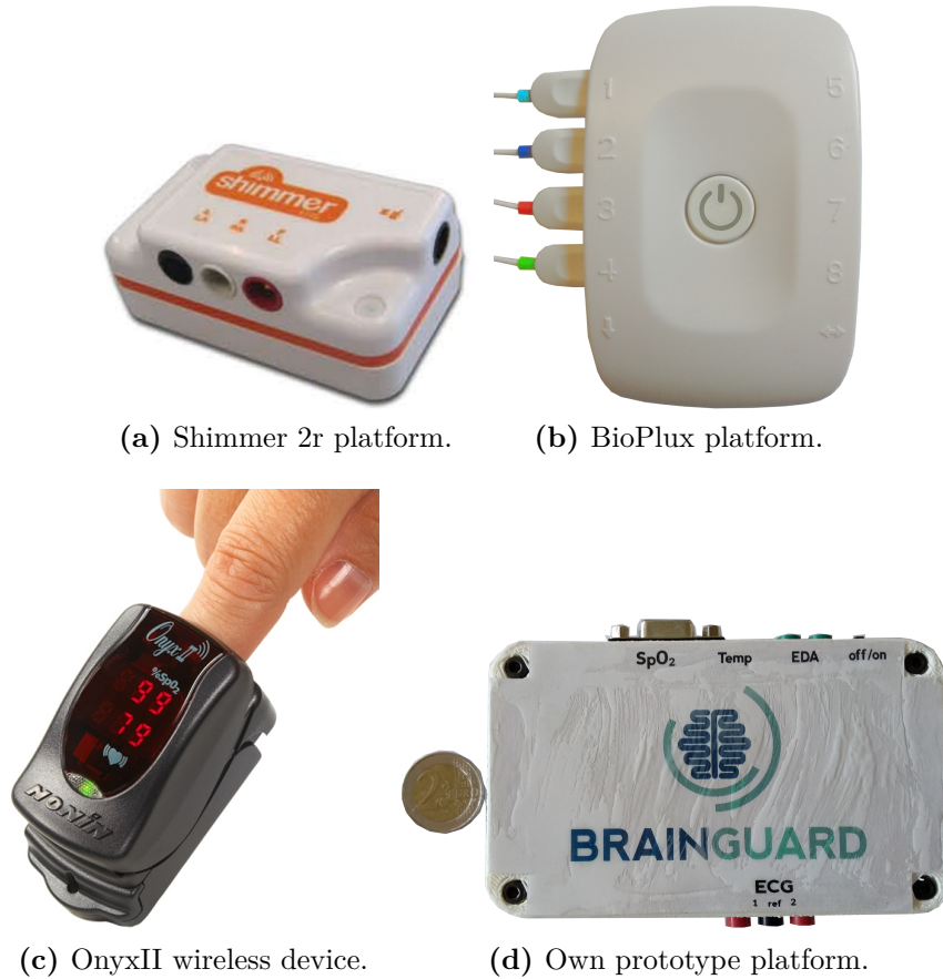
Figure 3.4: Different monitoring devices used along the implementation of the methodology to gather hemodynamic data and run fine-grained predictions.
