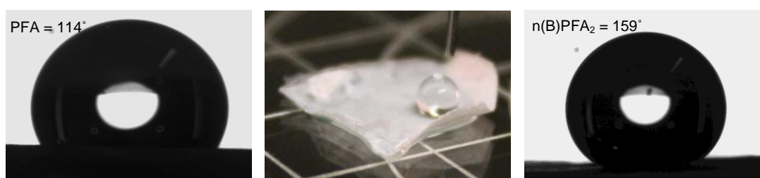
Figure 5.12. Hydrophobicity enhancement of the fluorinated surface (PFA) after nanostructuring by AAO templates.
