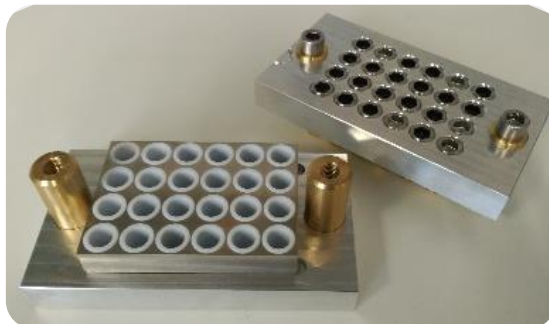
Figure 1. 4: High throughput solvothermal autoclave reactors at IMDEA Energy. 60
