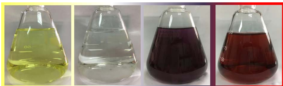
Figure 5. Evolution (from left to right) of the formation of AuNSs synthesized by the Turkevitch method.
