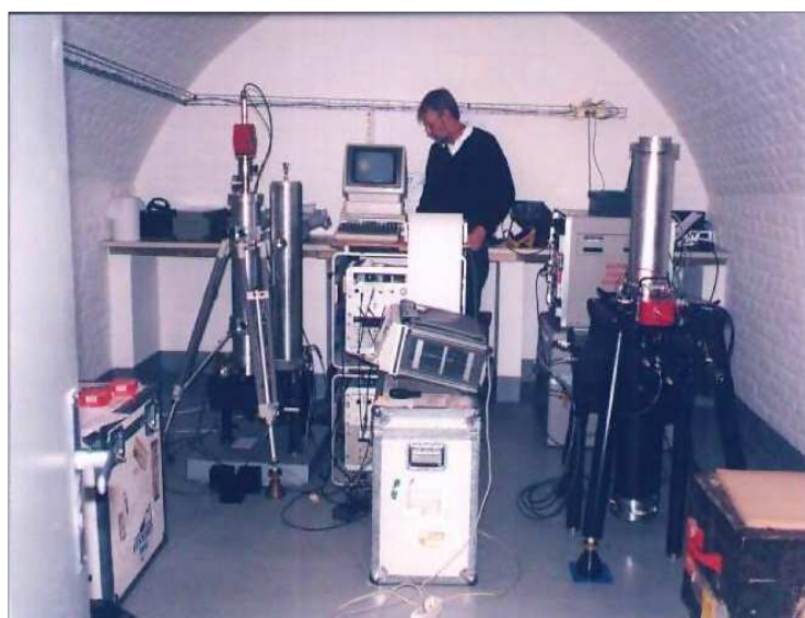
Fig. 3.11: Picture of both absolute gravimeter models, JILAg-5 and FG5#206 during the co-located measurement made in 1996 at J9 Observatory.
