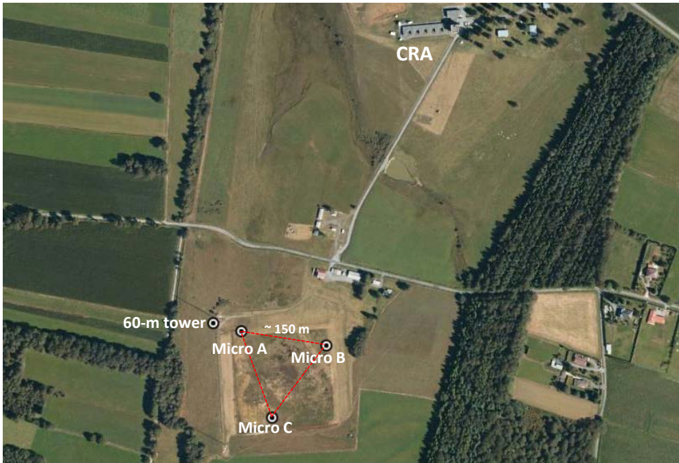
Figure 2.5: Location of three microbarometers during the BLLAST campaign at the CRA area.
