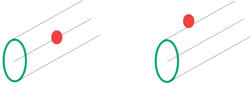
Figure 7.9: Sketch of a vacancy-DL interaction. On the left, the vacancy (red) is located inside the cylinder described by the radius of the DL (green) and its axis of motion (in the middle), and trapping may occur [14, 225, 236]. On the right, the vacancy is located on the edge of the cylinder, therefore both defects will recombine.
