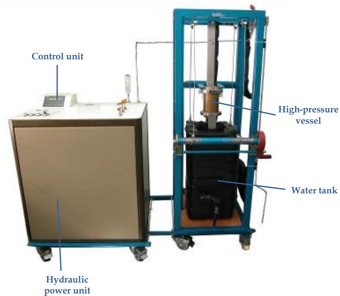
Figure 3.3. Lab-scale high-pressure equipment used for nearly-isothermal/isobaric experiments.
