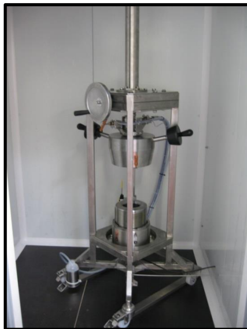
Figure 3.2. High-pressure stainless steel vessels used for hyperbaric storage in this work.
