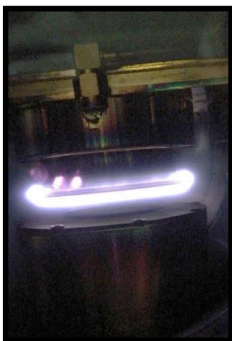
Figure 2.2: Oxygen plasma formed around a complex oxide target.
