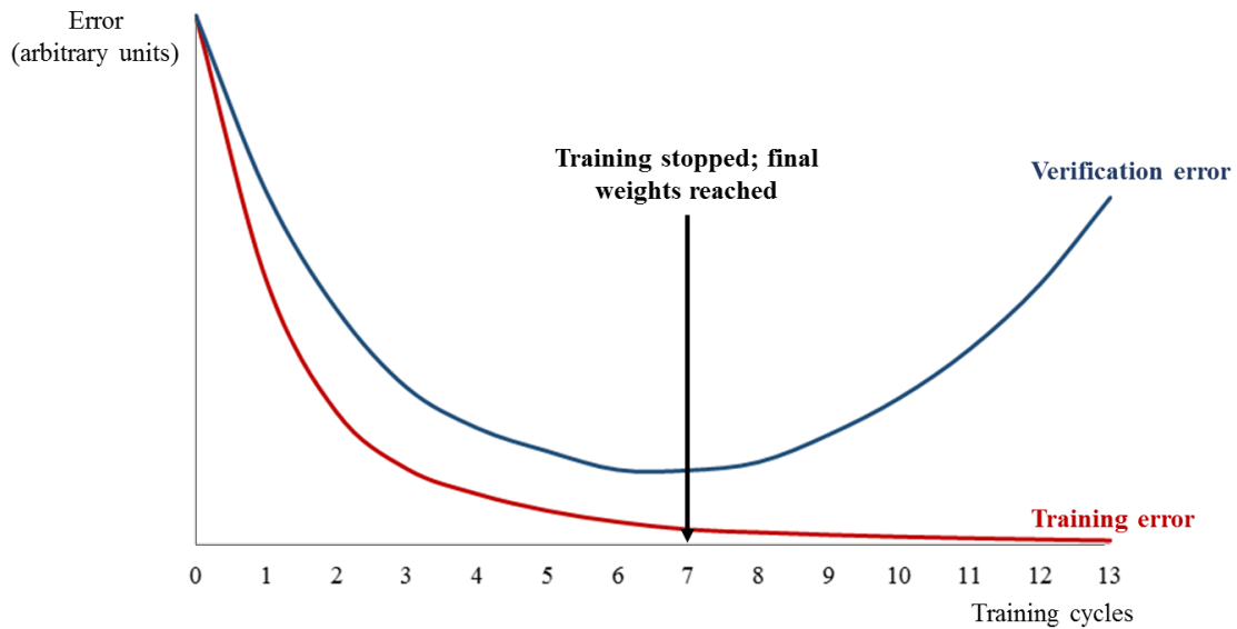
Figure 18. Chart that represents the typical development of the error concerning both datasets involved in the training process of a MLP: training dataset (red) and verification dataset (blue).
