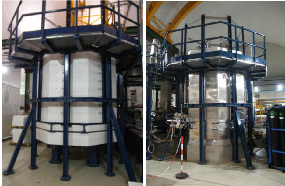
Figure 3.10: (Left) Lateral view of ArDM experiment showing the neutron shield already painted with fire retardant paint and before installing the outer fire protection layers. (Right) Lateral view of ArDM experiment showing the neutron shield with the outer fire protection already installed. The entire lateral surface is covered by two protection layers: an inner mineral wool thermal isolation sheet and the external aluminium layer.
