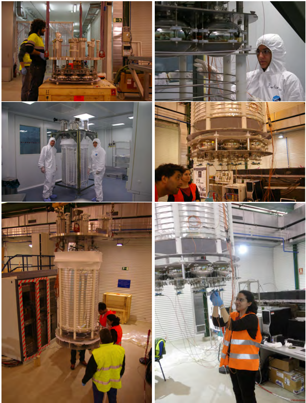
Figure 3.21: (Top left) Assembly of the top PMT array. (Top right) Installation of the field shapers, reflectors and top PMT connections inside the LSC clean room. (Middle left) Field cage completely mounted inside the clean room. (Middle right) Installation of the bottom PMT array. (Bottom left) Field cage hanging from the laboratory crane. (Bottom right) Connecting PMTs of the bottom array.
