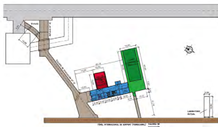
Figure 3.18: LSC installations located between an old railway tunnel and the Somport road tunnel. Hall A in which ArDM experiment is installed is depicted in green.
