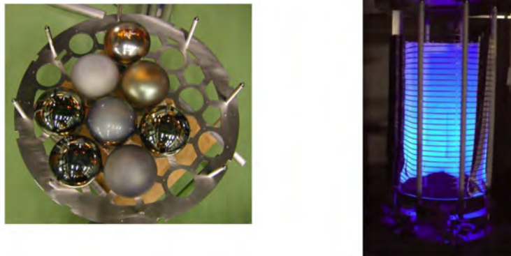
Figure 3.16: (Left) Top view of the temporary 7 PMT array used for the first measurements in liquid argon. (Right) TPB covered lateral TTX foils within the drift field shaper ring electrodes, illuminated with UV light.
