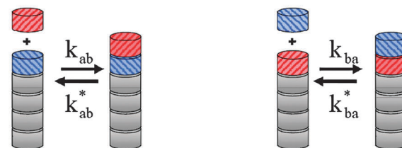
Fig. 1 The copolymerization model. The (R)-chiral (red) and (S)-chiral (blue) monomers reversibly associate into the growing homochiral (top) or heterochiral (bottom) copolymer chains. Because the system is closed , both the heterodimer (second line) and heterotrimer (third and fourth lines) reactions must be treated separately to avoid double counting and thus ensure that the total system mass is conserved in a closed system (see the text for an explanation).
